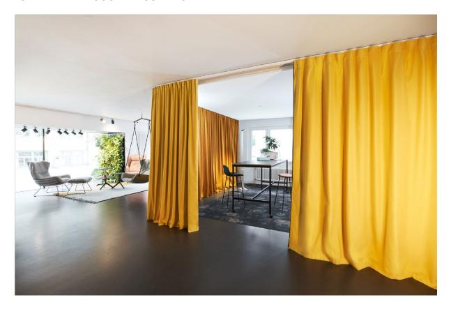
Création Baumann presents the highly functional ACOUSTIC DIVIDER VARIO system with the innovative NOISEBLOCKER technology for acoustically flexible room partitioning. For the ACOUSTIC DIVIDER VARIO with NOISEBLOCKER, Création Baumann uses a self-developed core made of synthetic rubber as a sound-absorbing membrane. Uniquely, the ACOUSTIC DIVIDER VARIO with NOISEBLOCKER achieves a reduction of 23 dB with only one inner layer and thus meets the requirements for highly effective sound insulation.
