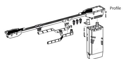
Robust extruded aluminium track suitable for heavy curtains, provided by electric motor, installed left or right as required:
