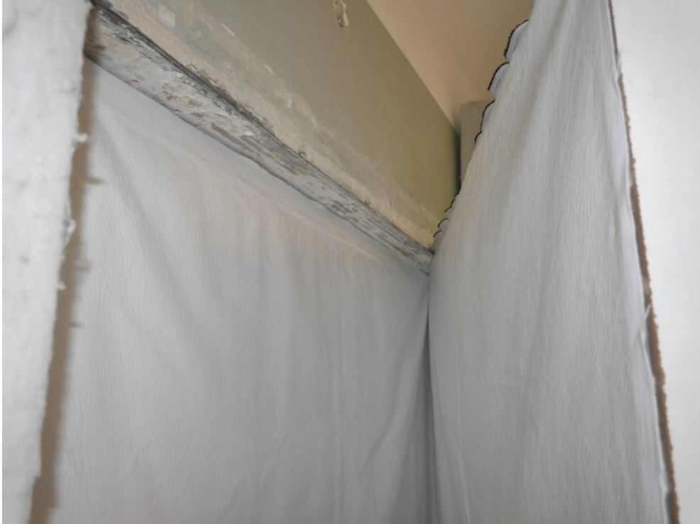
Figure B.4. Exemplary picture of a setup with two layers of molton/film in the window test stand (test setup opened).
